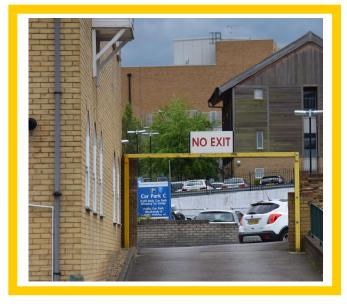
Height Restriction barrier is an effective method of preventing unauthorised access to any high sided vehicles such as truck and caravans. Manufactured from galvanised steel and painted finish to provide a durable and effective product. Optional extras available such as knocking bars, root fixed or surface fixed options.
