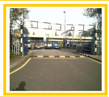
Heavy Duty Height Restriction Barrier and Swing Gate combination is a highly effective deterrent for both controlling access to the carpark, as well as limiting the type of vehicles entering the area. The swing gate can be locked to prevent all access to the car park when required and opened to allow low vehicles access. This is a very popular option with country parks, schools, and public carparks with limited opening hours.
