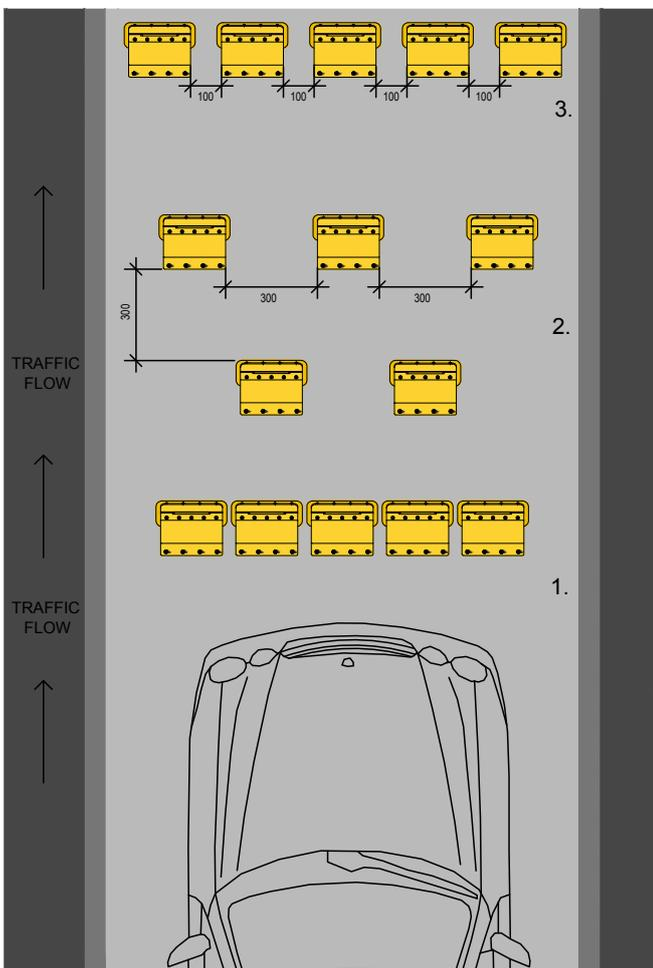
Note: All Flow Plates should be set out as shown in the diagram away from an area of turning
