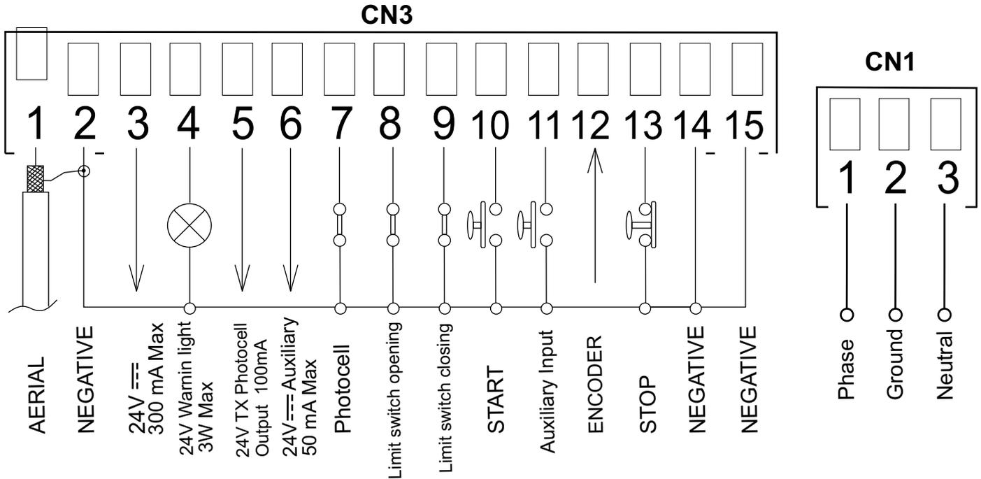
**Note 1:** The 24V=== Aux supplies 24V=== during the whole movement of the gate and during the pause when in automatic logic, while in semiautomatic logic only during the gate movement. On this output it is possible to connect a relay with 24V=== spool for the activation of a contact for generic use.
